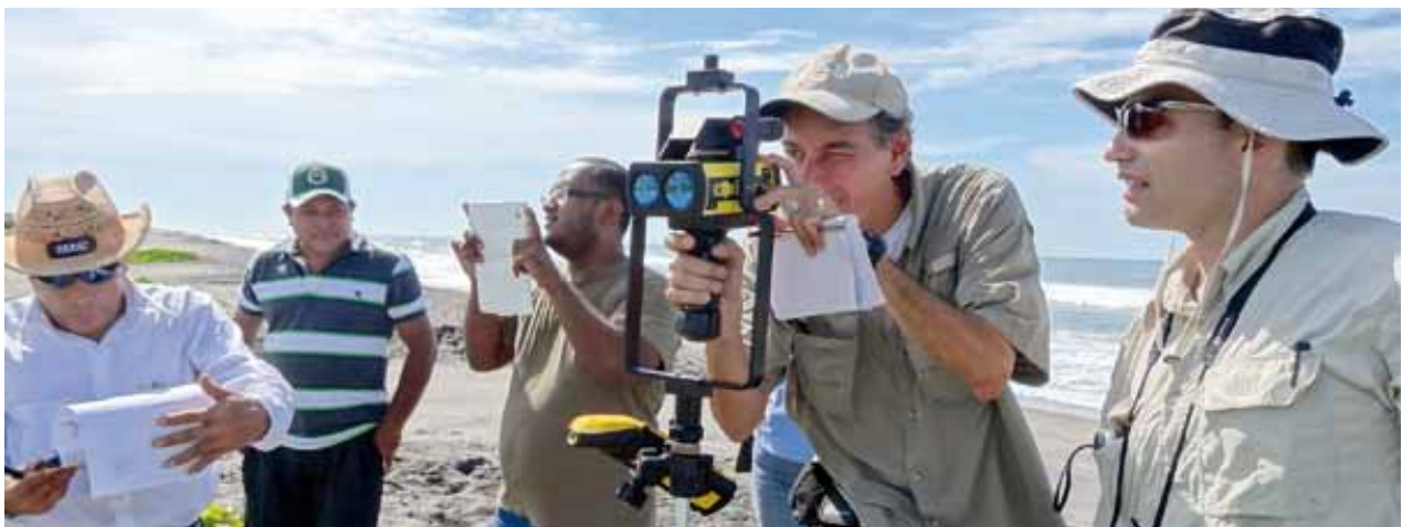
ITST measuring tsunami runup using laser rangefinder in El Salvador, 2012. Photo courtesy of ITIC
